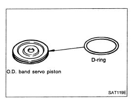
5. Remove O-rings from O.D. servo piston retainer.
