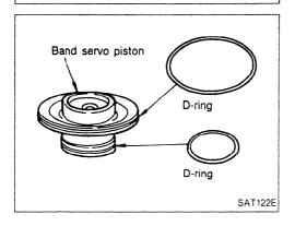
10. Remove D-rings from band servo piston.
