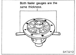
If not within specification, adjust clearance by changing thickness of side gear thrust washers.
