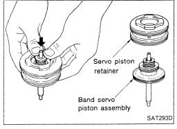
7. Place piston stem end on a wooden block. While pushing servo piston spring retainer down, remove E-ring.
