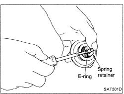
3. Place piston stem end on a wooden block. While pushing servo piston spring retainer down, install E-ring.
