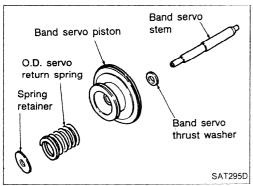
2. Install band servo piston stem, band servo thrust washer, O.D. servo return spring and spring retainer to band servo piston.
