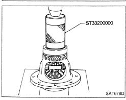
6. Press differential side bearings on differential case.
