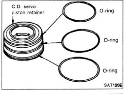
6. Remove band servo piston assembly from servo piston retainer by pushing it forward.
