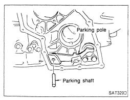
3. Install parking pawl on transmission case and fix it with parking shaft.
