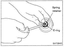
8. Remove O.D. servo return spring, band servo thrust washer and band servo piston stem from band servo piston.
