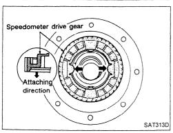
3. Remove speedometer drive gear.
