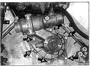
Remove fasteners A and B (arrows).
