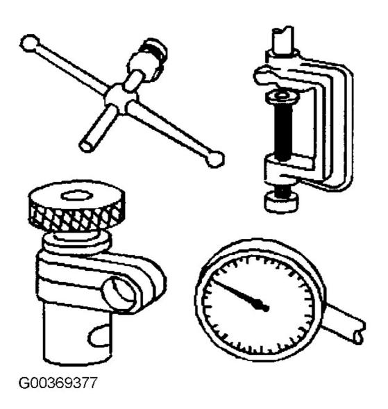
Fig. 3: Dial Indicator Set (J-8001) Courtesy of GENERAL MOTORS CORP.
