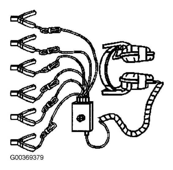
Fig. 4: Chassis Ear (J-39570) Courtesy of GENERAL MOTORS CORP.
