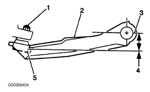
Fig. 2: Measuring Z Height Courtesy of GENERAL MOTORS CORP.
