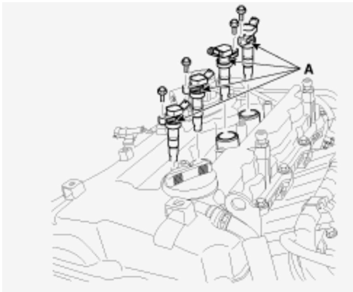
Fig. 6: Removing Ignition Coils (A) Courtesy of KIA MOTORS AMERICA, INC.
