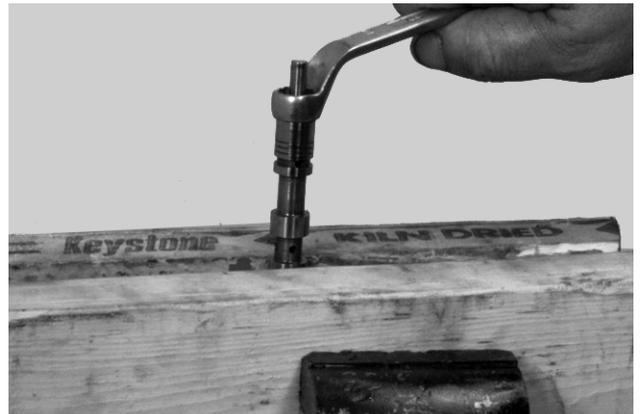
Put the spool (8) in a vice using wooden shims to protect the spool. Remove the cap screw (9) from the spool (8).
