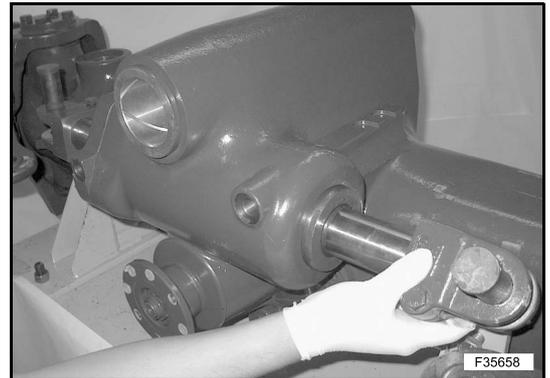
Once adjusted, tighten the nuts to the prescribed tightening torque of 117 Nm (86.3 lbf-ft).
