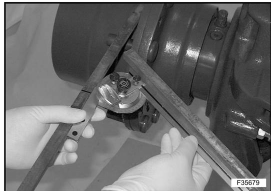
Adjust the mechanical steering stopper, by screwing in or out the relevant screws on the body, and then locking them by means of the lock nut.
