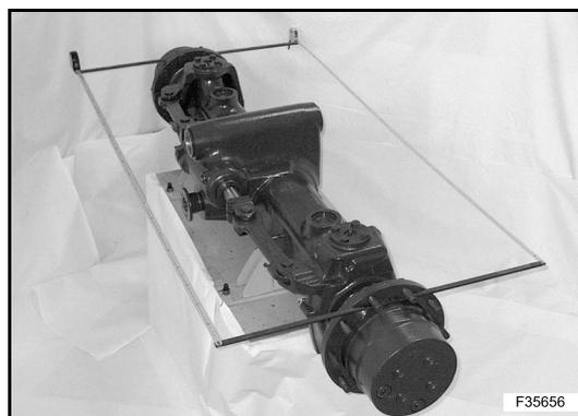
Check that the difference between the measurements at the ends of the wheel hub diameters is within the required tolerance range.
