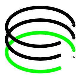
8. Fit the o-rings into the grooves in the cylinder liner. 84-engines, fit the o-rings into the grooves in the cylinder block. Fit the green o-ring (A) into the lowest groove. Lubricate the o-rings with a liquid soap (not with engine oil).
