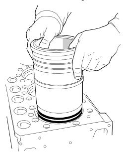
9. Press the cylinder liners into the cylinder block. It should be easy to press them fully home. Make sure that the liners do not rise up after fitting.
