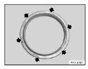
**Fig. 82: Locating Radial Seal** Courtesy of BMW OF NORTH AMERICA, INC.
