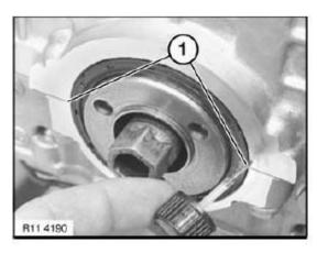
Fig. 78: Coating Surface Of Sealing Compound In Both Grooves With Loctite Primer Courtesy of BMW OF NORTH AMERICA, INC.
