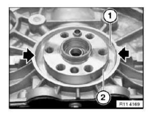
**Fig. 85: Identifying Sealing Cleaning Area And Radial Shaft Seal Running Surface Area** Courtesy of BMW OF NORTH AMERICA, INC.
