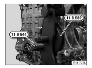
**Fig. 80: Positioning Special Tool (11 8 532) On Sealing Cover Courtesy of BMW OF NORTH AMERICA, INC.**
