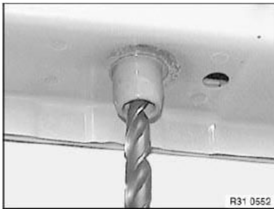
Fig. 7: Drilling Out Screw Remnants Courtesy of BMW OF NORTH AMERICA, INC.
