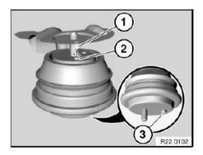
Fig. 2: Identifying Lug Of Heat Shield, Bore Of Engine Mount And Pin Courtesy of BMW OF NORTH AMERICA, INC.
