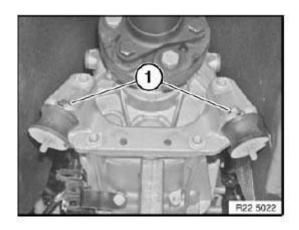
Fig. 9: Identifying Rubber Mount Screws
