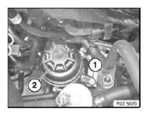
Fig. 7: Identifying Screws And Power Steering Expansion Tank Courtesy of BMW OF NORTH AMERICA, INC.
