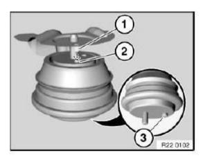
Fig. 4: Identifying Lug Of Heat Shield, Bore Of Engine Mount And Pin Courtesy of BMW OF NORTH AMERICA, INC.
