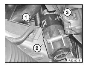
Fig. 5: Identifying Grounding Strap, Screws And VANOS Pressure Accumulator Courtesy of BMW OF NORTH AMERICA, INC.
