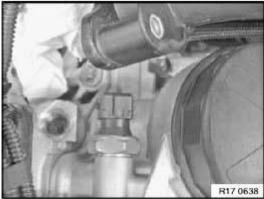
Fig. 3: Locating Mount Oil Pressure Switch On Filter Housing Courtesy of BMW OF NORTH AMERICA, INC.
