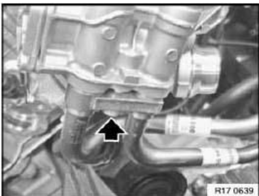
Fig. 4: Locating Mount Sealing Rings On Oil Supply And Return Lines Courtesy of BMW OF NORTH AMERICA, INC.
