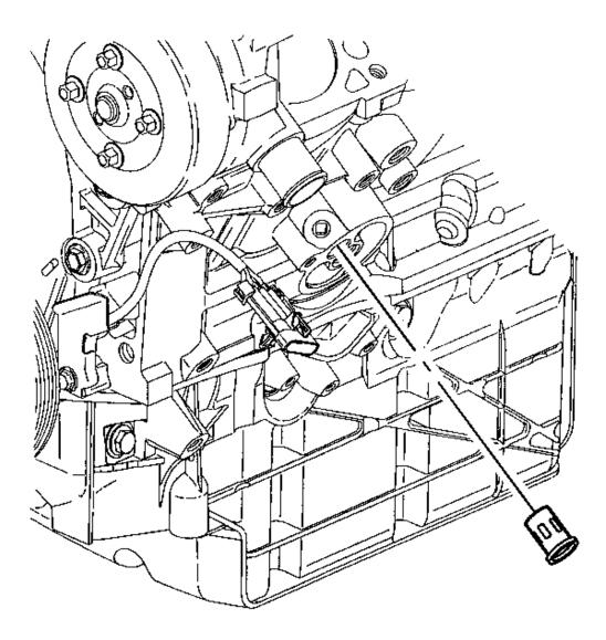
**Fig. 44: Oil Filter Bypass Valve** Courtesy of GENERAL MOTORS CORP.
