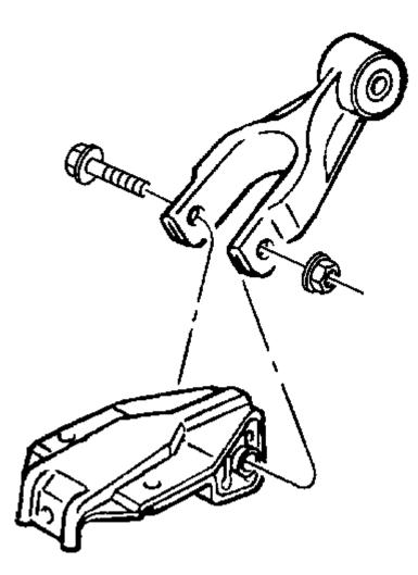
**Fig. 38: Engine Mount Strut** Courtesy of GENERAL MOTORS CORP.
