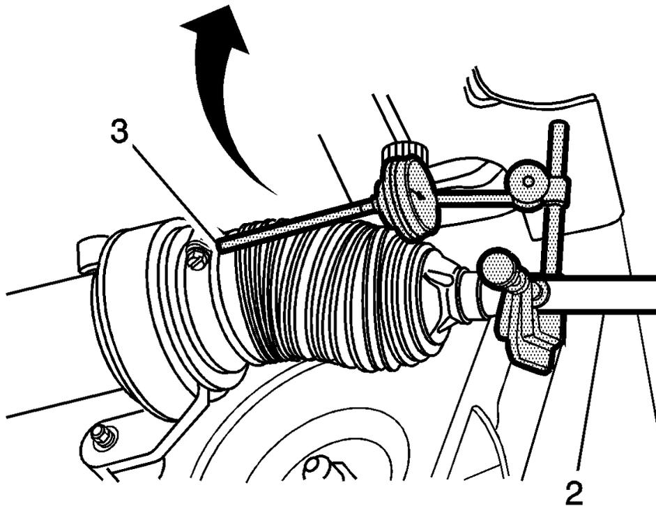
**Fig. 5: Measuring Lash Between Inner Tie Rod & Steering Gear Housing**
