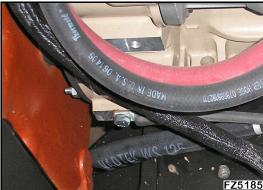
450FXL-1 50-133 ② 3. Remove 12 nuts (1) and washers (2) from studs (3).
