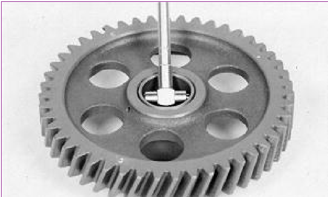
M35492-UN: Install Bushing Flush with Surface of Idler Gear
