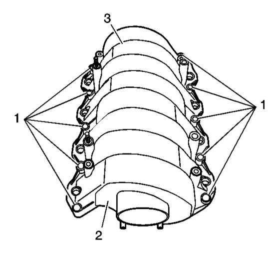
Fig. 117: Inspecting Intake Manifold For Cracks & Damage To Bolt Bosses Courtesy of GENERAL MOTORS CORP.
