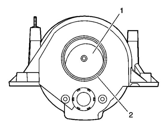
Fig. 119: Inspecting Front Intake Manifold For Damage To Passage & Plenum Duct Neck Courtesy of GENERAL MOTORS CORP.
