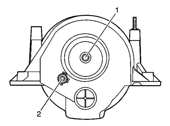
Fig. 120: Inspecting Intake Manifold For Damage To PCV System Hose & Vacuum Ports Courtesy of GENERAL MOTORS CORP.
