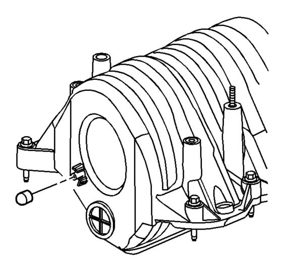
Fig. 115: View Of Vacuum Cap Courtesy of GENERAL MOTORS CORP.
