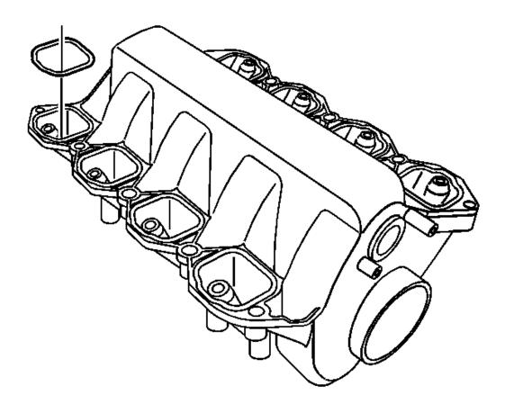
Fig. 122: View Of Intake Manifold-To-Cylinder Head Gaskets Courtesy of GENERAL MOTORS CORP.
