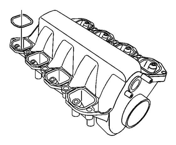
Fig. 114: View Of Intake Manifold-To-Cylinder Head Gaskets Courtesy of GENERAL MOTORS CORP.
