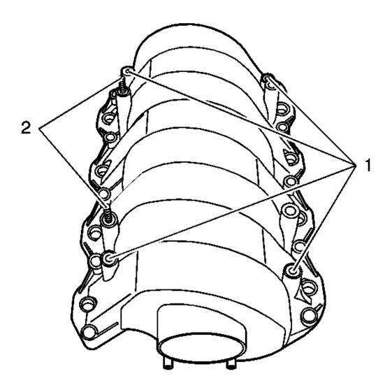
Fig. 116: Inspecting Intake Manifold For Damage To Fuel Rail Mounting Inserts & Studs Courtesy of GENERAL MOTORS CORP.
