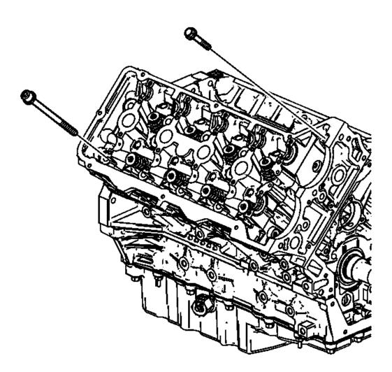
Fig. 2: View Of Right Cylinder Head Bolts
