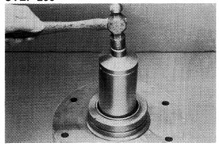
Push the oil seal into position using CAS 1465-2 driver.
