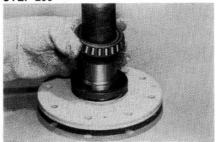
Remove the protective sleeve. Put the heated bearing on the axle shaft, the bearing must make contact with the shaft shoulder.
