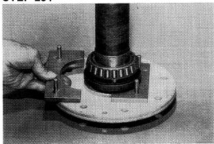
Install two CAS 1465-4 oil seal drivers under the oil seal.
