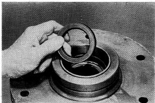
Put the inner oil seal in the axle housing.
