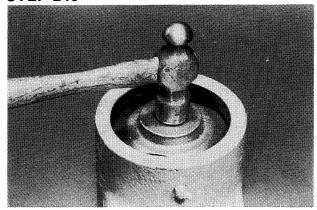
Install the axle housing outer bearing cup until the bearing is seated against the housing shoulder.
