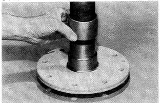
Stand the axle shaft on end and put the protective sleeve CAS 1465-4 on the axle shaft.
