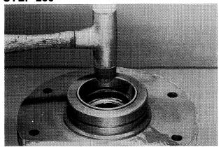
Install the axle housing inner bearing cup until it is seated against the housing shoulder.
