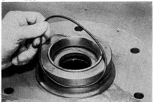
Install a new o-ring in the axle housing groove. Lubricate the o-ring with Case FDL oil.
