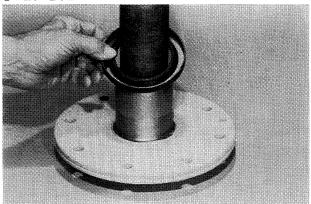
Press a new seal (lip up) over sleeve and on the axle shaft.
