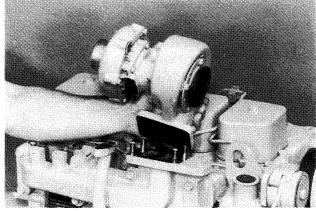
Install the turbocharger on the exhaust manifold.
