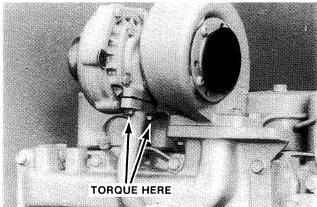
Tighten the oil drain tube bolts to a torque of 18 lb ft (24 Nm)(2.4 kgm).
