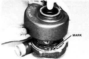
Install the turbine housing assembly on the compressor housing. Make sure the mark on the center housing is in align with the mark on the compressor housing.
