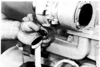
Install a new gasket on the oil drain tube.
