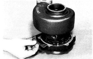
Install the compressor housing mounting plates.
