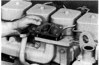
Install a new gasket on the exhaust manifold.
