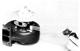
Install the new turbine housing bolts and tighten to a torque of 96 lb inch (11 Nm)(1.1 kgm).
