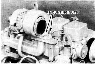
Install the turbocharger mounting nuts and tighten to a torque of 24 lb ft (32 Nm)(3.2 kgm).
