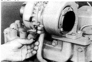
Install the oil drain tube bolts.
