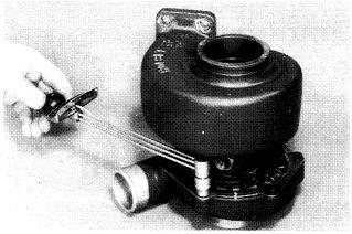
Install new lock washers and bolts in the compressor housing. Tighten the bolts to a torque of 48 lb inch (6 Nm)(0.6 kgm).
