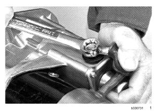
2. Loosen and remove the screws that mount the cover to the brush holder.
