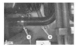
6. Loosen clamp (10), and disconnect lower radiator hose (11) from the radiator.
