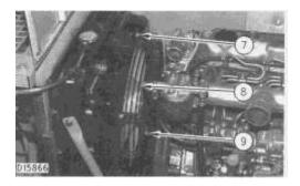
5. Loosen two bolts (9). Remove three bolts (7) and the washers. Remove upper fan guard (8).
