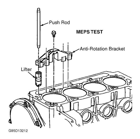
Fig. 7: Identifying Push Rod, Anti-Rotation Bracket & Lifter Courtesy of GENERAL MOTORS CORP.
