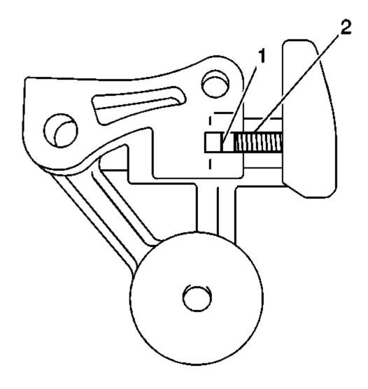
Fig. 80: View Of Timing Chain Tensioner Latch & Teeth Courtesy of GENERAL MOTORS CORP.
