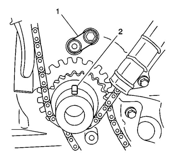
Fig. 81: View Of Crankshaft Keyway Courtesy of GENERAL MOTORS CORP.
