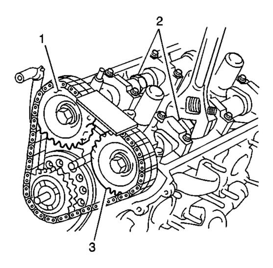
Fig. 78: View Of Camshaft & Sprockets Courtesy of GENERAL MOTORS CORP.
