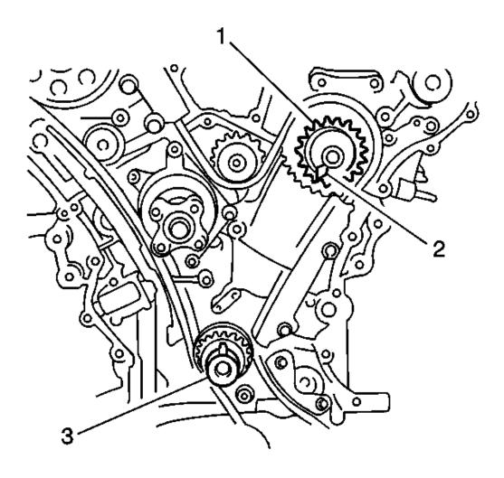
Fig. 82: View Of Idler Sprocket & Timing Mark Courtesy of GENERAL MOTORS CORP.
