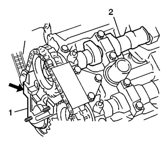
Fig. 77: View Of Timing Chain Tensioner & Intake Camshaft Courtesy of GENERAL MOTORS CORP.
