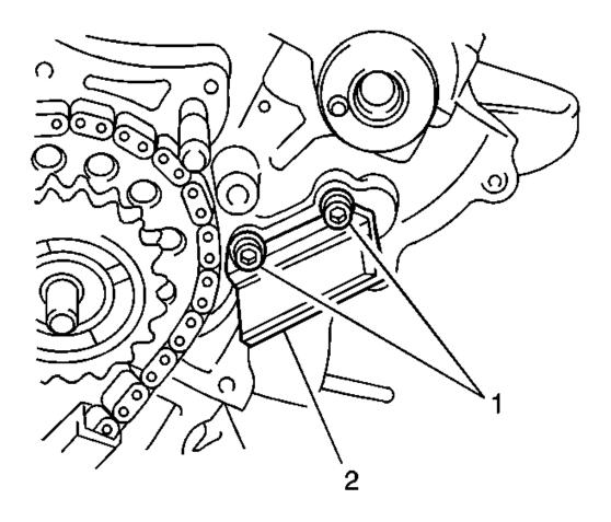
Fig. 79: View Of Side Chain Guide & Bolts Courtesy of GENERAL MOTORS CORP.
