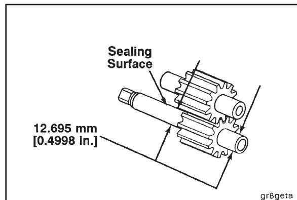
Visually inspect the gears for damage and replace them if needed. Check the gear width. Discard any gear worn smaller than 31.707 mm [1.2483 in].
