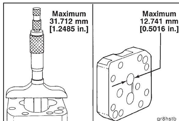
Check the shaft bores in the cover and the body.
