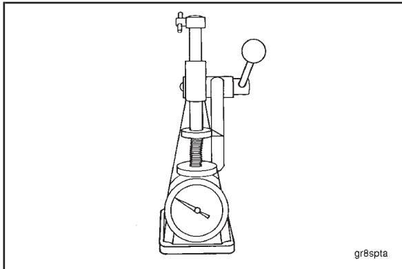
Inspect the regulator spring for damage and replace if needed. The spring **must** meet the specifications as shown in the table.
