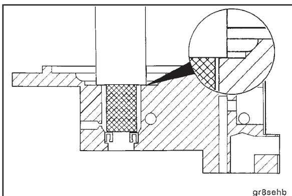
Install the fuel seal first. This is the seal nearest to the gear pump. The seal lip **must** be toward the gear pump.
