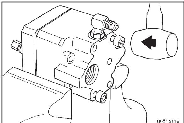
Clamp the gear pump housing in a vise. Gently tap alternately on the head of the capscrews to loosen the gear pump cover.
