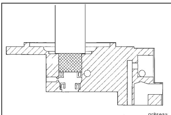
Install the oil seal. The seal lip **must** be away from the gear pump side.
