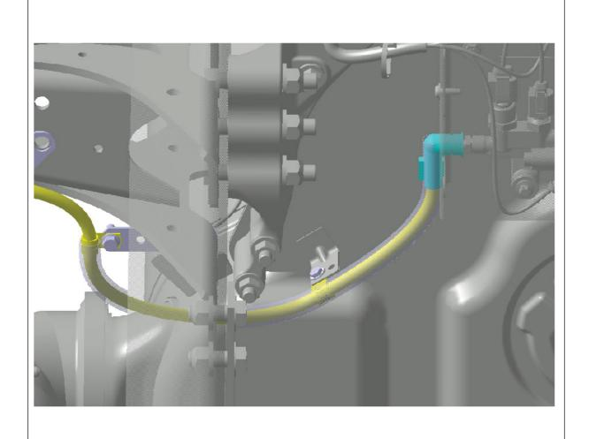
5. Connect the compressed air line connection (1) to the DEF metering unit by pushing it into the "quick-connect" connection.
