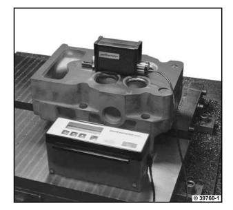
Measure cylinder head height with depth measuring appliance.
