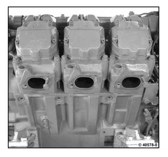
• Remove rocker arm and rocker arm bracket.
