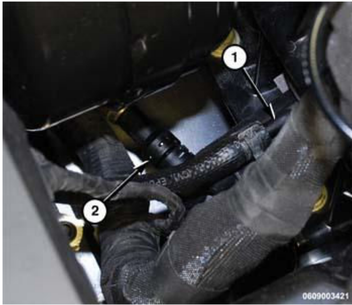
Fig. 18: Peak Torque Limiter & Pressure Hose Courtesy of CHRYSLER GROUP, LLC
