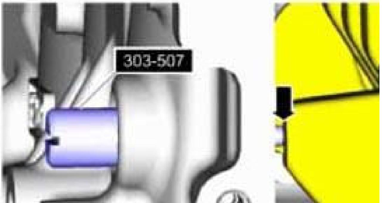
9. **NOTE:** The Camshaft Alignment Timing Tool is for camshaft alignment only. Using this tool to prevent engine rotation can result in engine damage.
