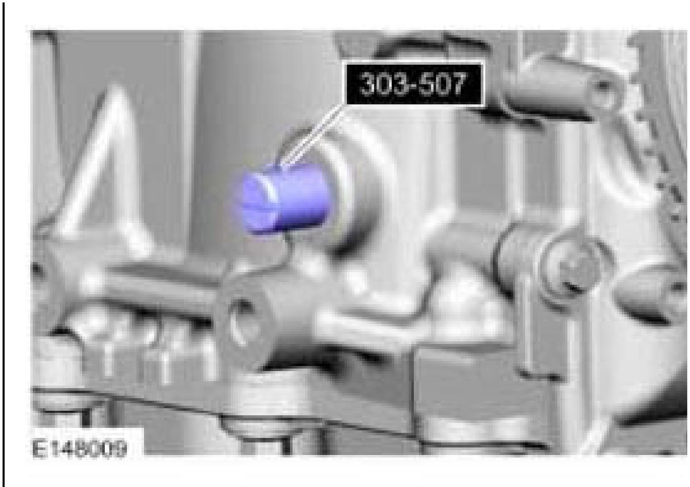
8. **NOTE:** The Crankshaft TDC Timing Peg will contact the crankshaft and prevent it from turning past TDC. However, the crankshaft can still be rotated in the counterclockwise direction. The crankshaft must remain at the TDC position during the crankshaft pulley removal and installation.
