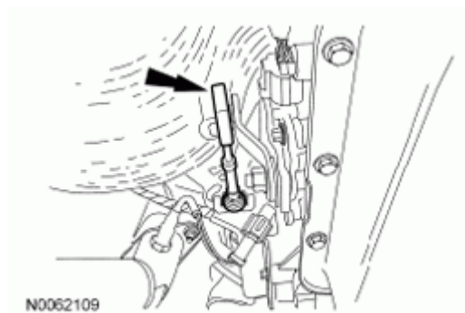
Fig. 22: Locating Selector Lever Cable Courtesy of FORD MOTOR CO.
