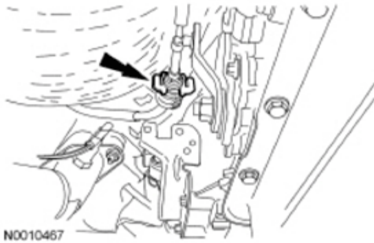
Fig. 23: Locating Selector Lever Cable Retaining Clip Courtesy of FORD MOTOR CO.
