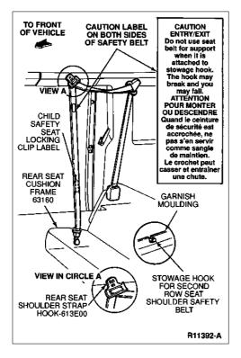
Rear Safety Belt Assembly, Three-Passenger, Aerostar
