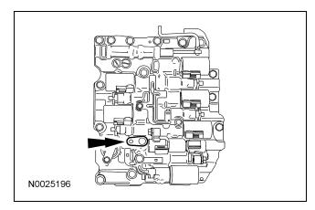
The transmission fluid temperature sensor, which is integrated within the transmission wiring, is installed on the front of the valve body. It directs the fluid temperature within the hydraulic pressure control circuit and transmits a signal based on that temperature to the TCM. Through this it controls gear shift, lockup and slip in response to changes in fluid temperature for smooth shifting across wide fluid temperature zones.
