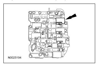
The torque converter clutch (TCC) solenoid is used in the transaxle control system to control the application, modulation and release of the torque converter clutch.
