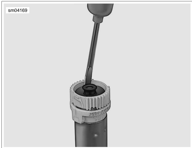
Figure 4-22. Install Seal Cap If Removed
