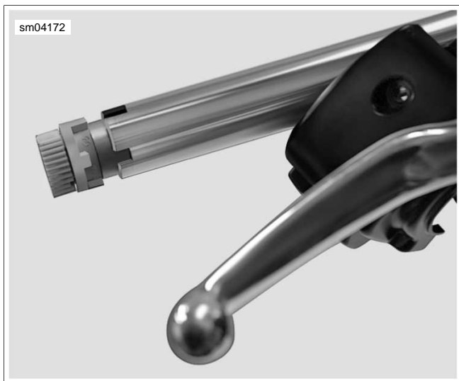
Figure 4-23. Install Twist Grip Sensor
