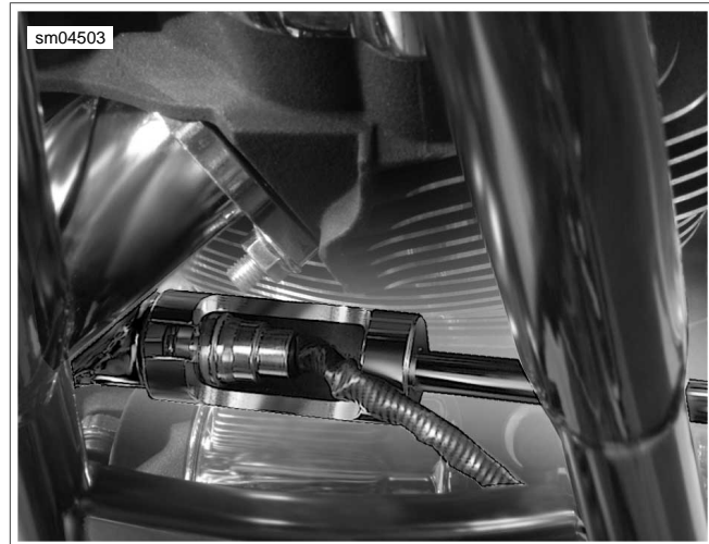
Figure 4-31. Remove/Install Front O2 Sensor
