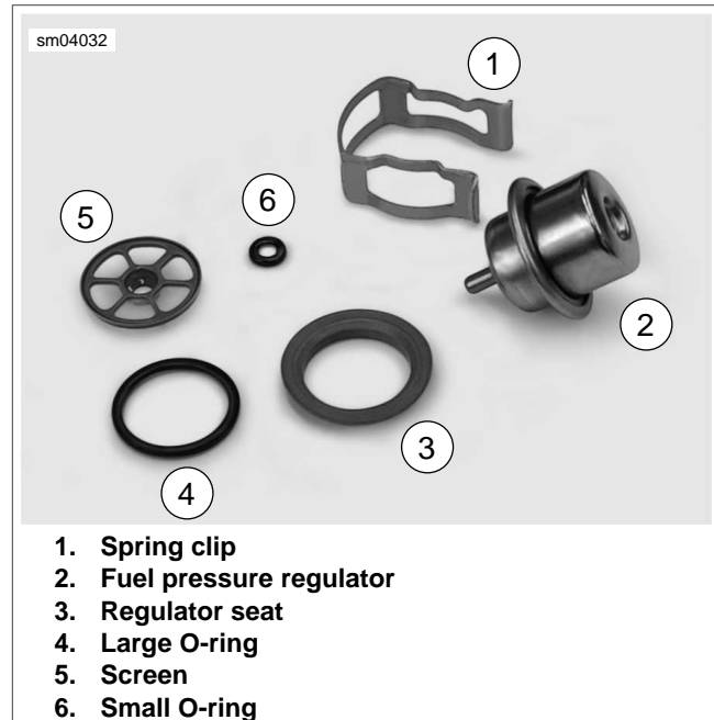
Figure 4-15. Fuel Pressure Regulator Assembly
