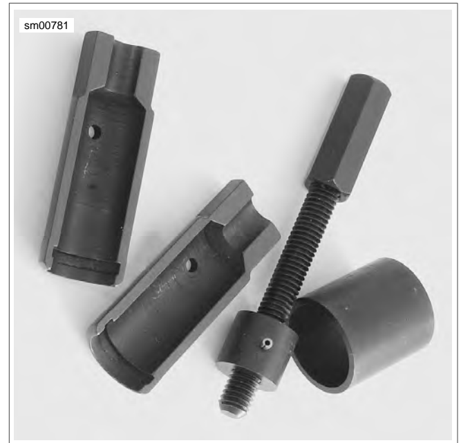
Figure 7-80. Counterbalancer Bearing Inner Race Remover and Installer (HD-46582)
