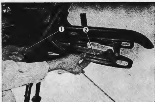
Fig. 4.62 Removing the rear fork
