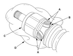
4. Make marks (A) on the rollers (B) and the spider (C) to identify the locations of the rollers on the spider, then remove the rollers.
