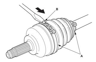
2. Slide the outboard boot (A) partially to the inboard joint side. Be careful not to damage the boot.
