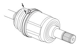
17. Bend the band end (A) by tapping it down with a hammer.
