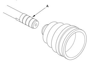
2. Install the inboard boot onto the driveshaft, then remove the vinyl tape. Be careful not to damage the inboard boot.
