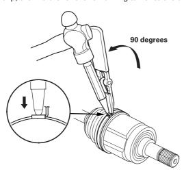
16. Unwind the boot band tool, and cut off the excess free end of the band to leave a 5—10 mm (0.2—0.4 in.) tail protruding from the clip.
