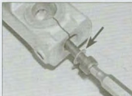
7.7 Remove the damper rod bolt and sealing washer (arrowed)
