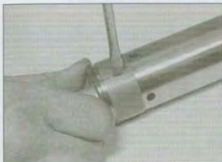
7.17 Prise the bottom bush apart with a flat-bladed screwdriver and slide it off the end of the tube
