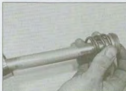
7.8 Withdraw the damper rod and rebound spring from the tube
