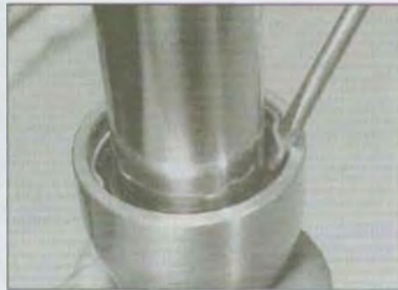
7.10 . . . then carefully remove the oil seal retaining clip
