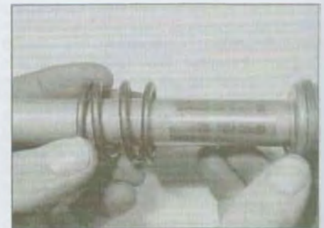
7.19a Slide the rebound spring onto the damper rod
