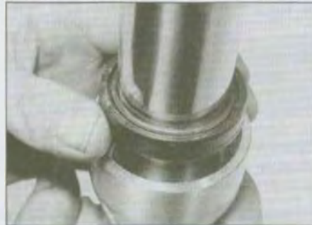
7.22 Install the oil seal with markings facing up
