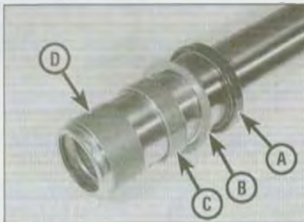
7.12 Oil seal (A), washer (B), top bush (C) and bottom bush (D)
