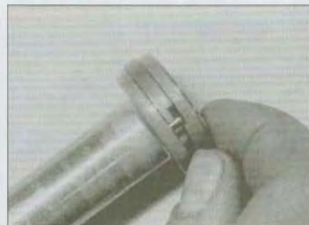
7.18 Renew the damper rod piston ring if it is worn or damaged
