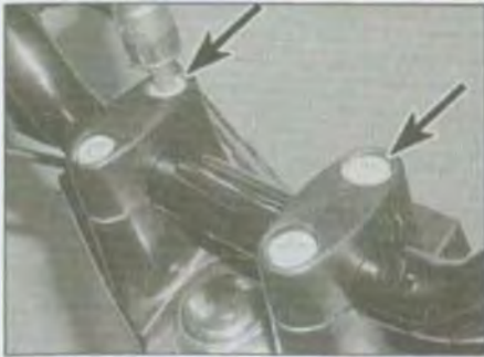
5.10a Tighten the front bolts (arrowed) first
