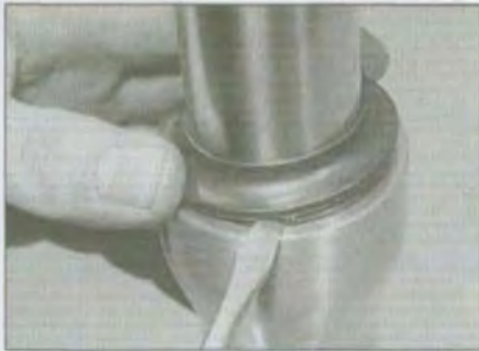
7.9 Prise out the dust seal . . .
