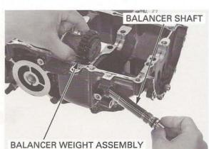
Turn the balancer shaft and position the punch mark on the shaft facing down.
