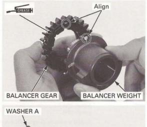
Apply oil to the needle bearing and install them into the balancer weight. Install the washer A and B as shown.
