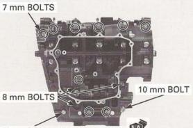
7 mm BOLT/SEALING WASHER
