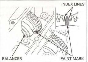
Install the lower crankcase onto the upper crankcase while aligning the crankshaft balancer drive gear white paint mark with between the balancer gear index lines as shown.
