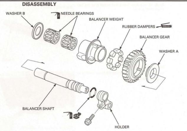
Apply grease to the damper rubber fitting area. Install the damper rubbers into the balancer gear. Assemble the balancer gear and weight while aligning the marks.
