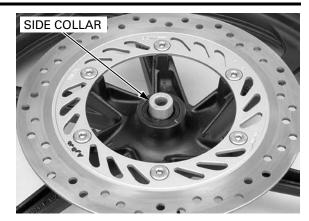
When installing the front wheel, align the following:
