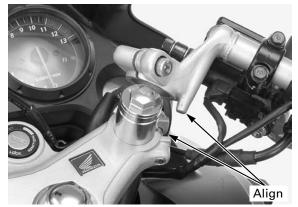
Tighten both handlebar pinch bolts to the specified torque.
