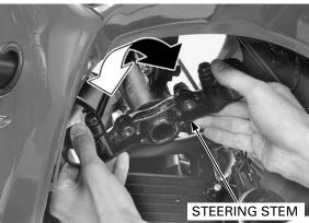
Retighten the adjusting nut to the specified torque using a special tool.
