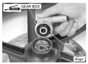
Install the side collar into the right wheel hub.
