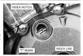
The index lines on the cam sprockets must be flush with the cylinder head surface as shown.
