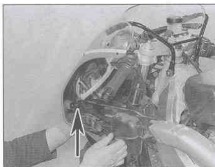
5.11b ... and remove the fairing, noting how the trim panels locate at the front (arrowed) ...
