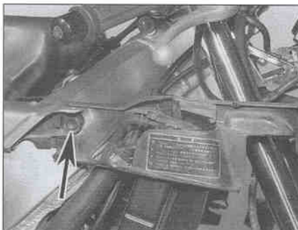
5.20a Remove the trim clip (arrowed) to release the front trim panel
