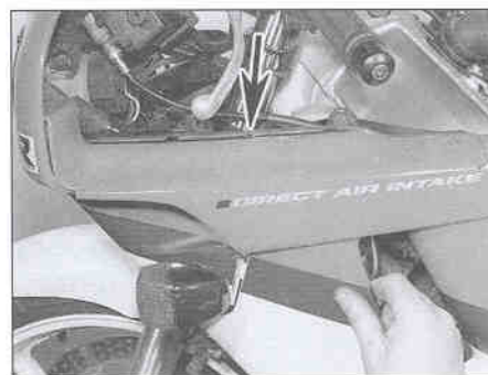
5.14b ... and lift the top off the locating pin (arrowed)
