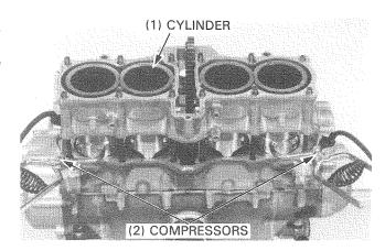
Install the cylinder bolt and tighten it securely.
