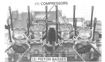
Attach the piston ring compressors to the No. 1 and No. 4 pistons
