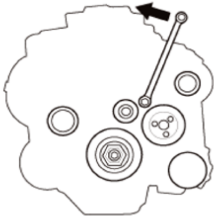
Fig. 2: Compressing Auto-Tensioner Courtesy of AMERICAN HONDA MOTOR CO., INC.
