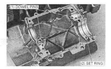
Install the mainshaft and countershaft by aligning the countershaft bearing groove with the set ring on the crankcase, and aligning the bearing cap holes with the dowel pins.
