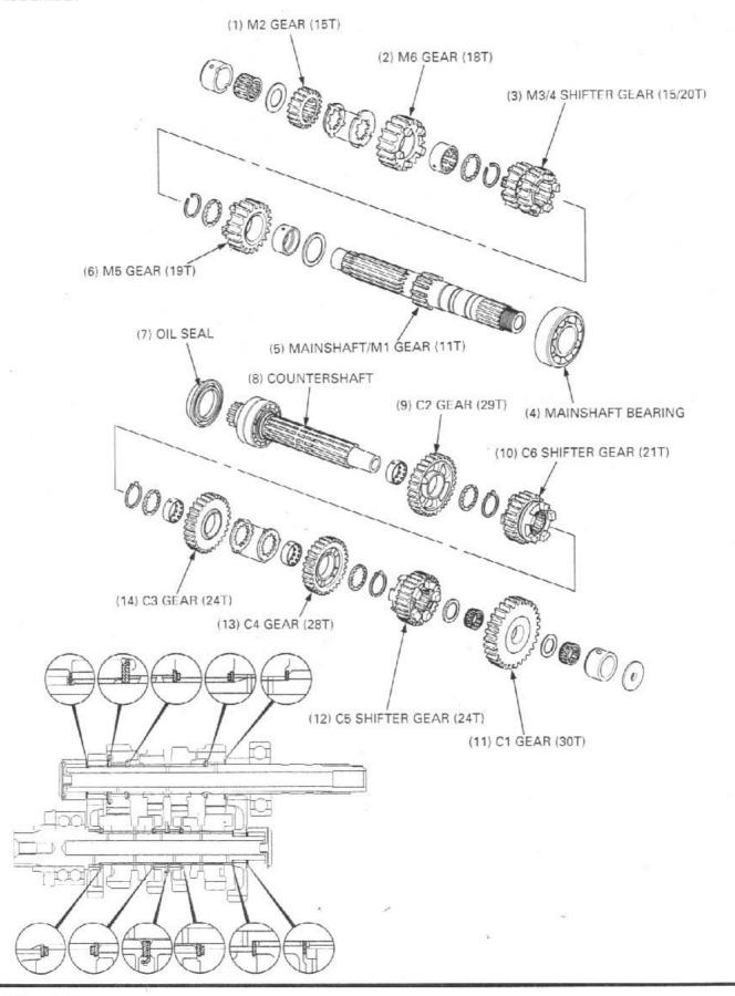
Assemble the transmission gear and shafts, Coat each gear with clean engine oil and check for smooth movement.
