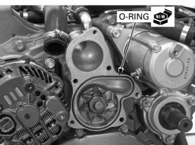
Install a new rubber seal onto the thermostat flange. Install the thermostat into the water pump cover with the hole facing upward while aligning the lug with the cover groove as shown.
