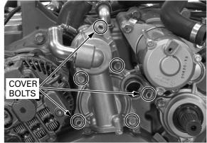
Install the water pump cover onto the pump. Install the three cover bolts and three mounting bolts, and tighten them.
