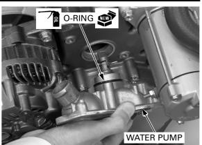
Install a new O-ring onto the water pump groove.
