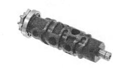
Turn the outer race of the shift drum bearing with your finger.
