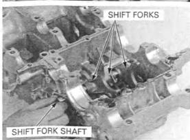
Remove the shift drum assembly.
