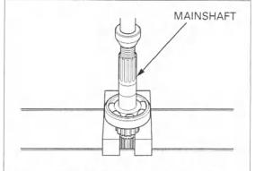
Install with the Install a new mainshaft bearing onto the mainshaft groove side facing by pressing the mainshaft bearing inner race using up. the special tools.
