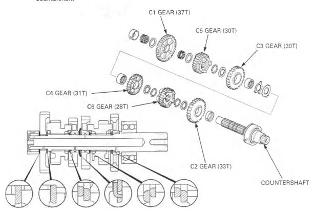
Assemble the transmission gear and shafts. Coat each gear with clean engine oil and check for smooth movement.
