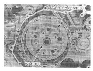
Remove the thrust washer.
