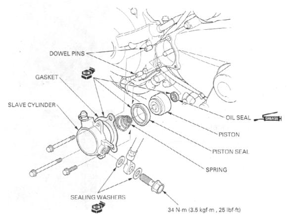
Apply small amount of silicone grease to the lifter rod contacting area of the piston.
