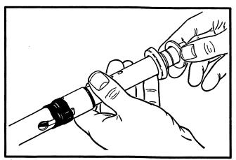
6. Apply a small amount of grease to the face of the retainer plate (36) and washer (35). Install the retainer plate and then the washer. The flange of the retainer plate must be towards the washer.
