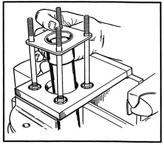
3. Apply clean grease to the bushing (38) and install the jacket tube assembly (37) on the service assembly fixture. Make sure that the square shoulder of the bolts engage the square holes in the upper cover.
