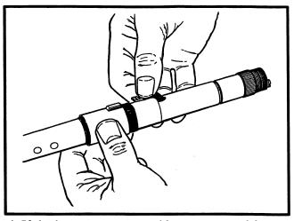
4. If the horn contact assembly was removed for repairs, install the horn contact assembly (43) on the input shaft. Make sure the position is like unit before it was disassembled.
