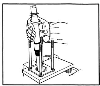
8. Slide the input shaft assembly into the upper cover and tube assembly.
