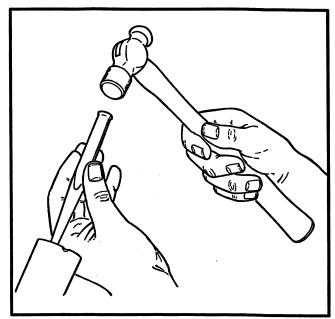
2. Use pliers or a punch to bend two small areas of the tube to lock the bushing in position. Do not use the original areas that were used as the locks.
