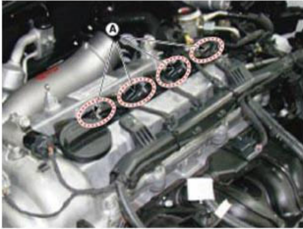
Fig. 4: Identifying Ignition Coil Connector Courtesy of HYUNDAI MOTOR AMERICA
