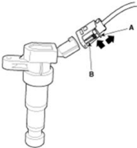
Fig. 5: Removing Ignition Coil Connector Courtesy of HYUNDAI MOTOR AMERICA
