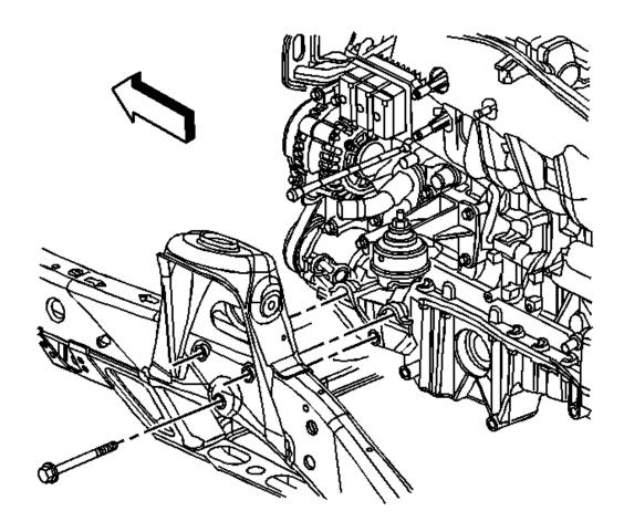
Fig. 59: View Of Left Frame Engine Mount Bracket Bolts Courtesy of GENERAL MOTORS CORP.
