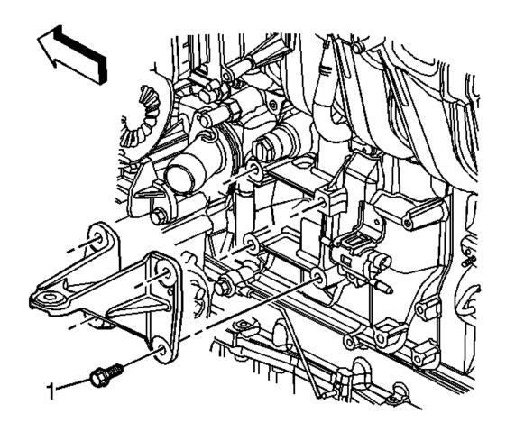
Fig. 60: View Of Left Engine Mount Bracket Bolts Courtesy of GENERAL MOTORS CORP.
