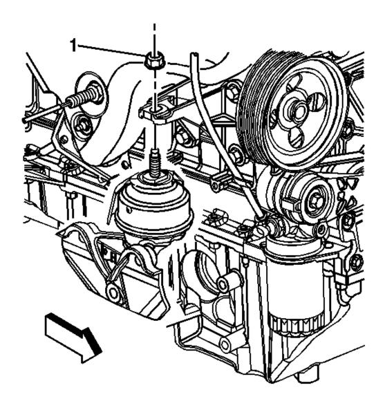
Fig. 61: View Of Upper Engine Mount Nuts Courtesy of GENERAL MOTORS CORP.
