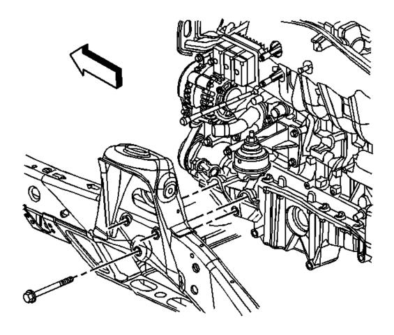
Fig. 58: View Of Left Frame Engine Mount Bracket Bolts Courtesy of GENERAL MOTORS CORP.
