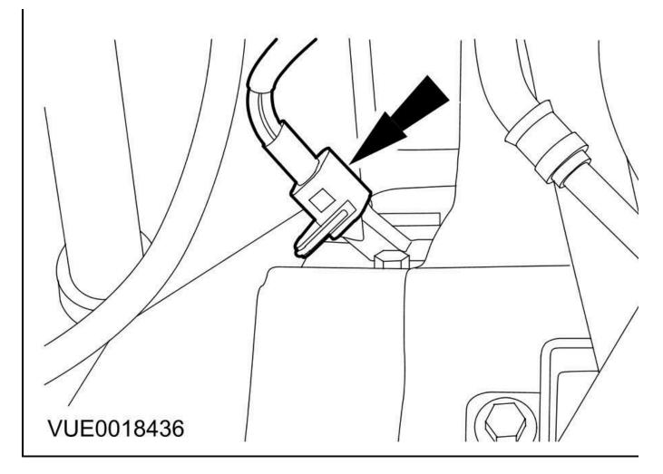
95. Disconnect the crankshaft sensor electrical connector.
