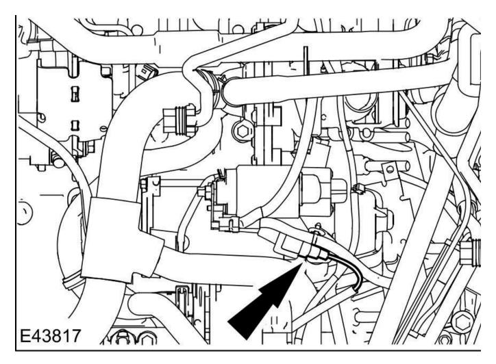
92. Disconnect the starter motor wiring harness electrical connector.
