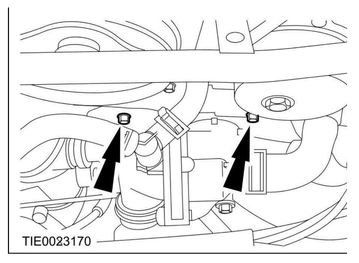
96. Remove the transmission upper retaining bolts.
